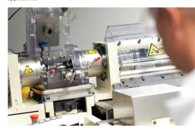
Our thrust-washer testing machines include thermal management to actively control temperature - by cooling and heating - to 200°C at the frictional interface. We have also increased their mechanical stability to drastically improve accuracy on measurements such as temperature sweeps, sliding speed sweeps or wear rate runs, and we've added the ability to measure wear and friction in lubricated conditions to meet the increased demand for application knowledge in lubricated systems.
